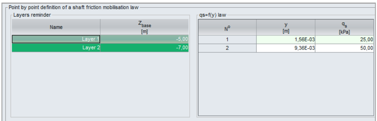
Figure F.22 : "Shaft friction mobilisation law definition" box – Point by point input
